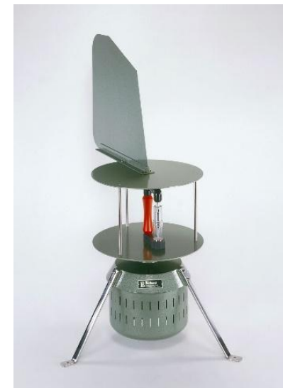
Cyclone sampler (Burkard Manufacturing Co Ltd) Projet Lifeplan
