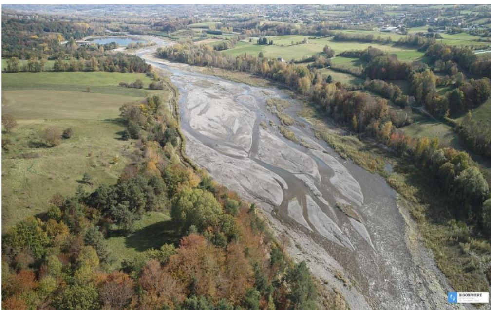
Drone view of the restored reach of the Upper Drac in 2018, showing the spontaneous recovery of the braided channel morphology (@SIGosphere)
